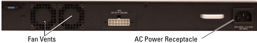
Figure 1-4. N1500 Series Back Panel
