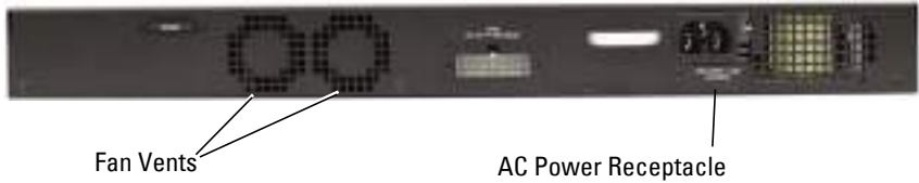
Figure 3-7. Dell EMC Networking N1500 Series Back Panel
