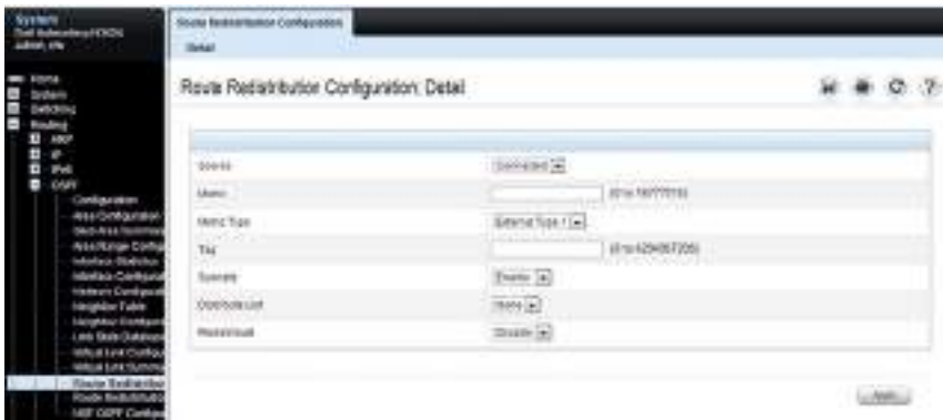
Figure 34-15. OSPF Route Redistribution Configuration
