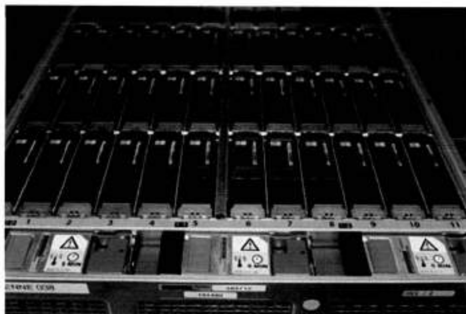
Figure 172. Fans and disk drives inside the disk enclosure
