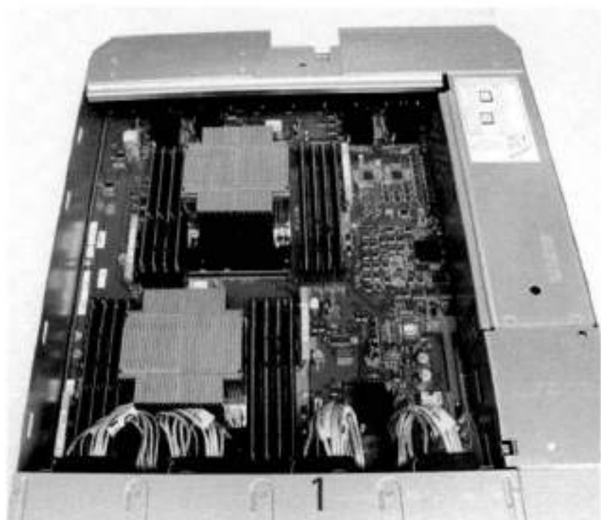
Figure 99. Top view of SP module with SP cover removed
